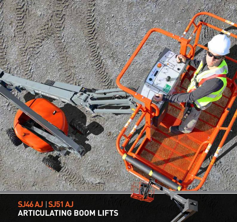
Skyjack's Articulating Boom Lifts are available in two models featuring the SJ46 AJ and SJ51 AJ. Both models boast an industry leading, standard equipped, 360 degree continuous turret rotation. Zero tail swing compliments the turret design allowing for flexible operation in tight locations. Superior positive traction and terrainability is provided by the axle based 4WD used in many of Skyjack's product designs, which accounts for a proven low maintenance, rugged and reliable drive train.
